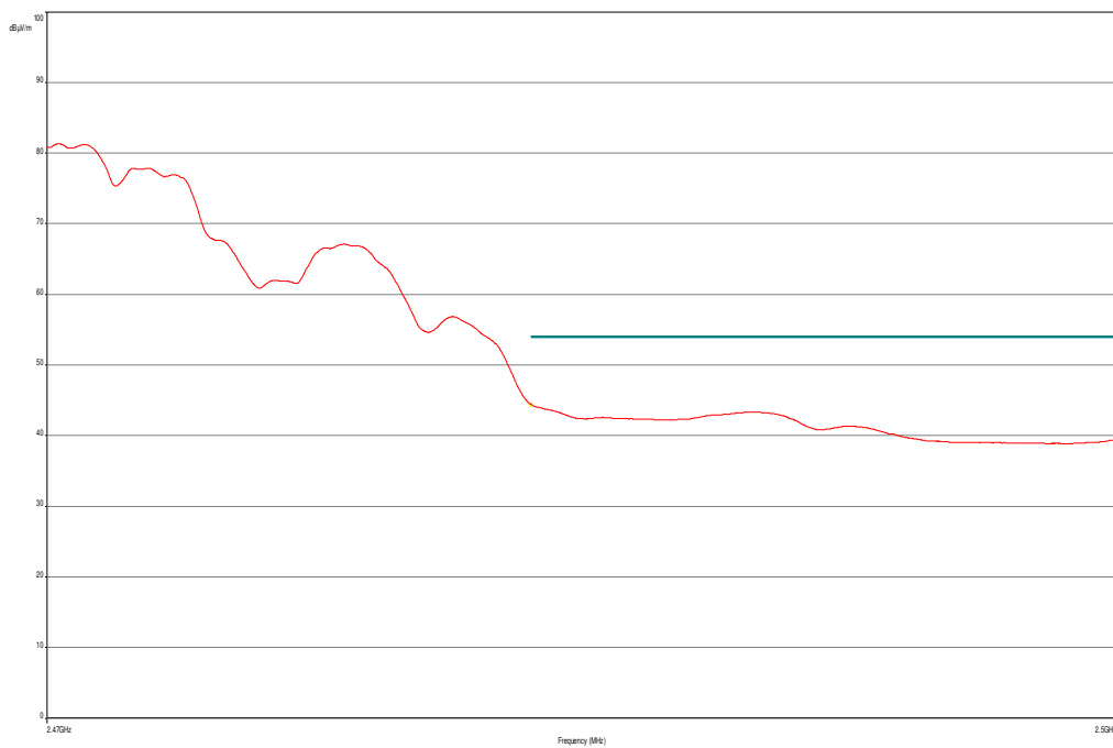
Plot 2: TX mode, upper band edge, vertical & horizontal polarization
