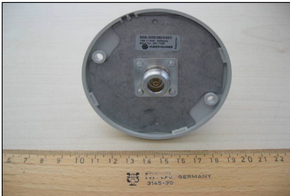
Photo 32: Omnidirectional antenna (CA Q14)
