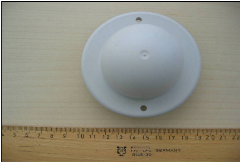
Photo 31: Omnidirectional antenna (CA Q14)
