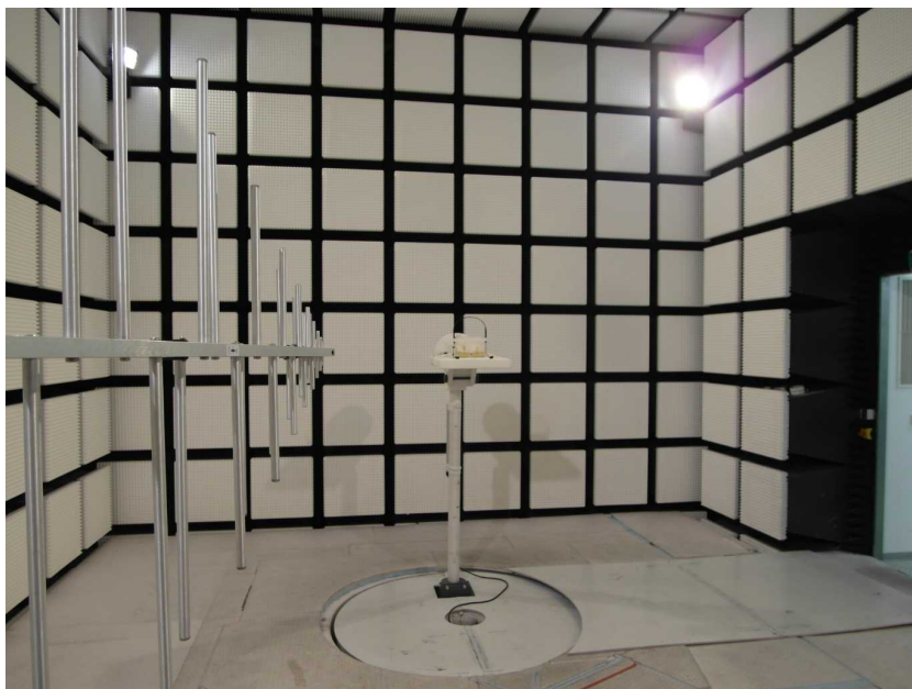
Photo 4: EUT at the anechoic chamber
