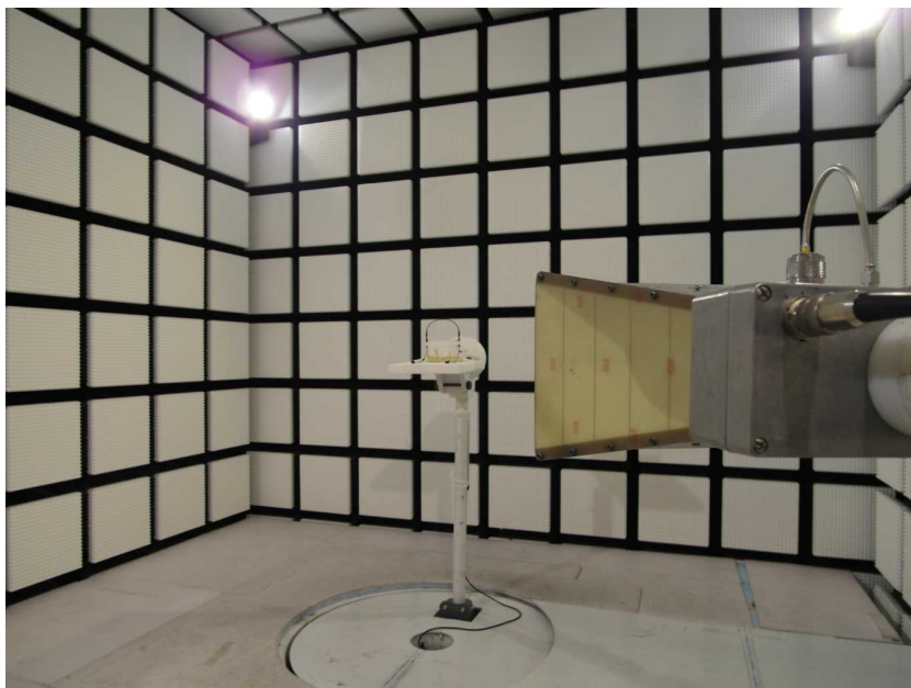
Photo 6: EUT at the anechoic chamber
