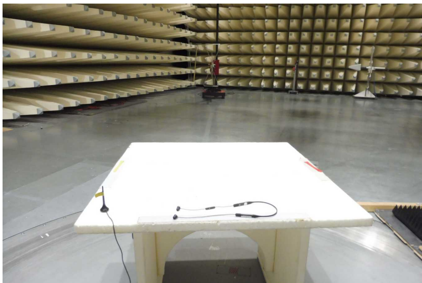
Photo 8: EUT at the semi-anechoic chamber
