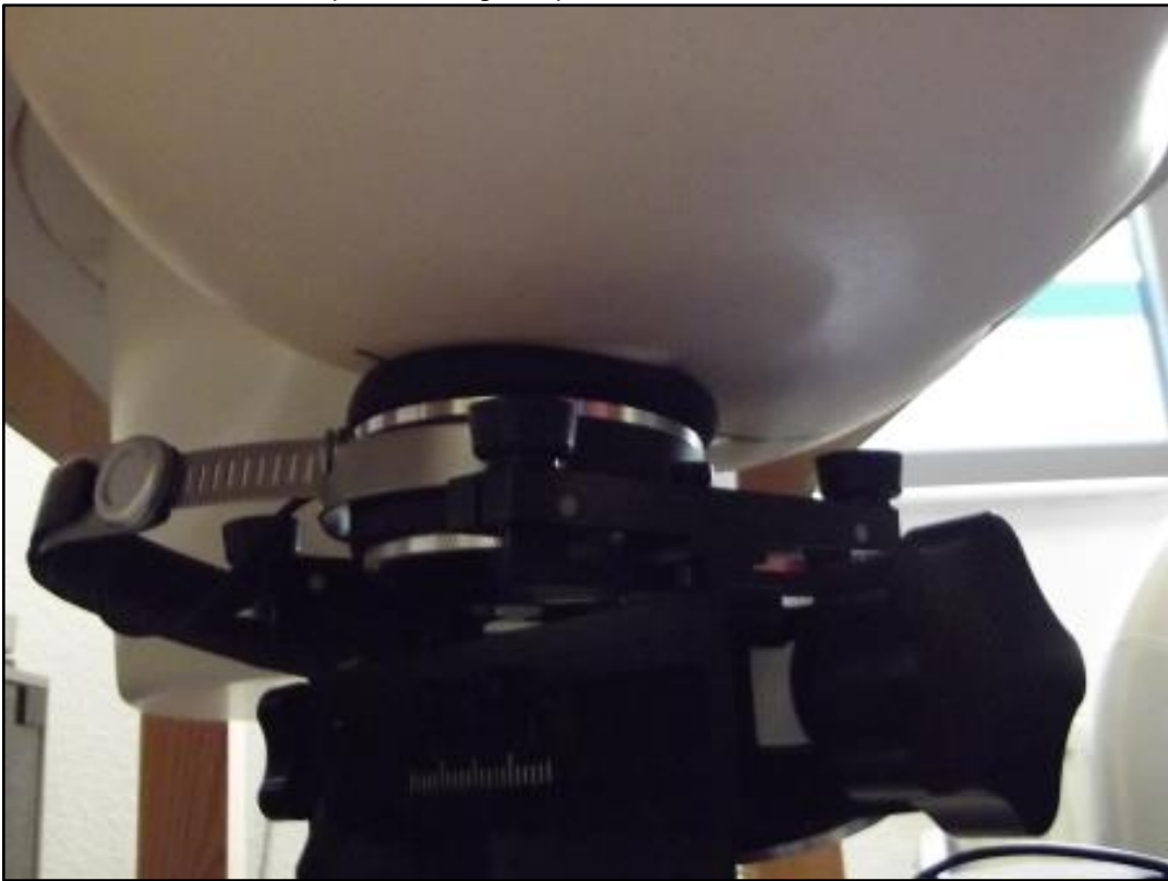
Photo 7: Test position - right capsule to the head with 0mm distance
