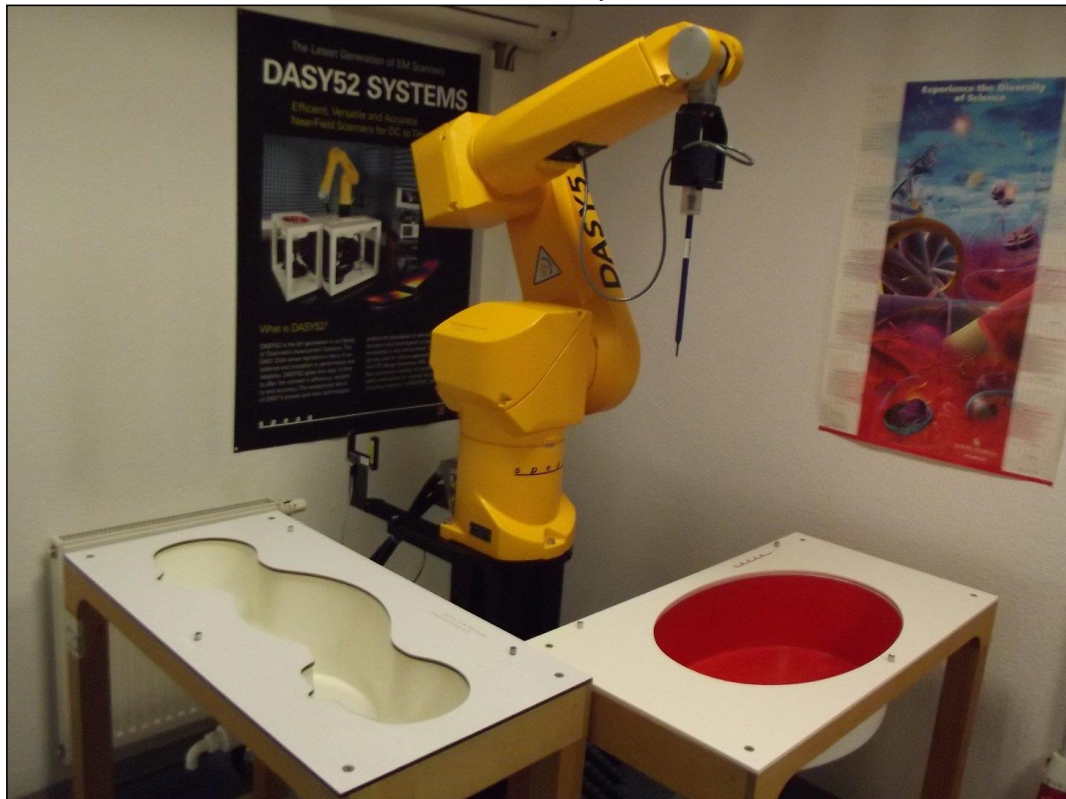
Photo 1: Measurement System DASY 5
