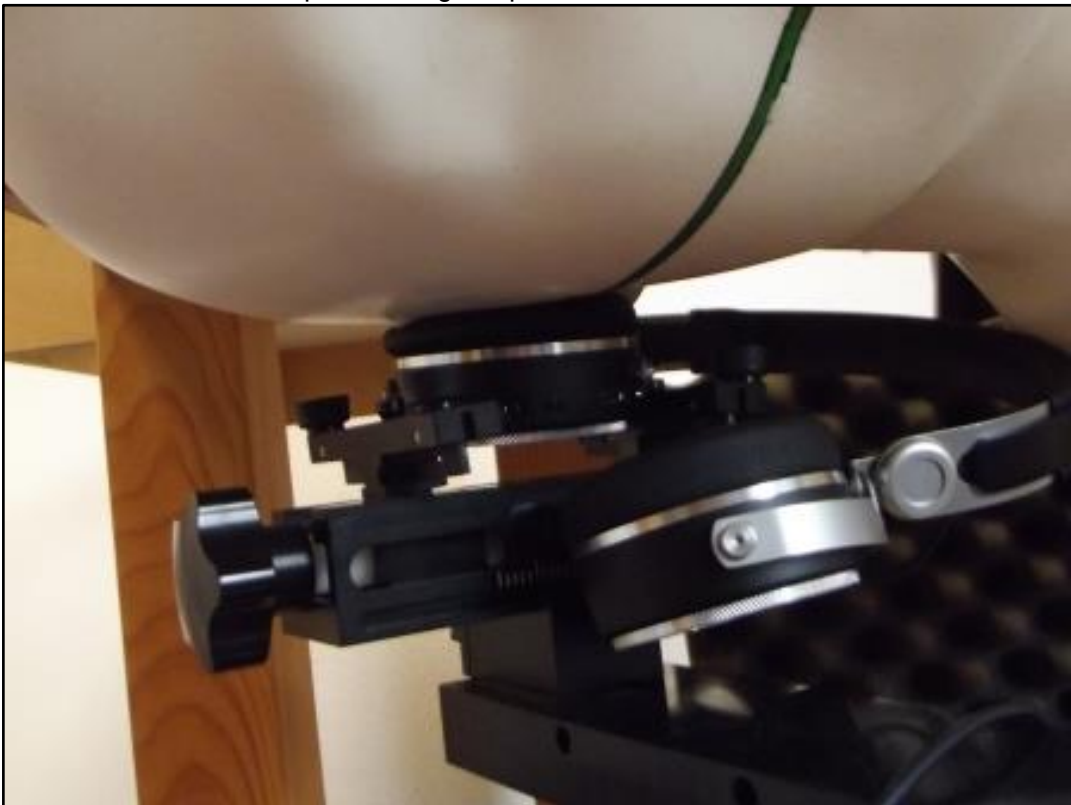
Photo 6: Test position - right capsule to the head with 0mm distance
