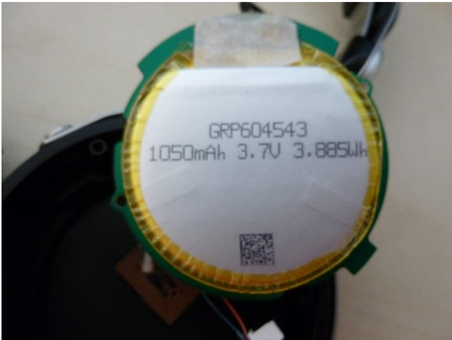
Photo 10: PCB 1 back side view (battery pack)
