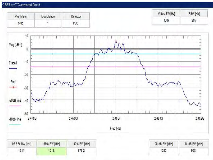
Plot 6: highest channel – 2480 MHz, Pi / DQPSK modulation
