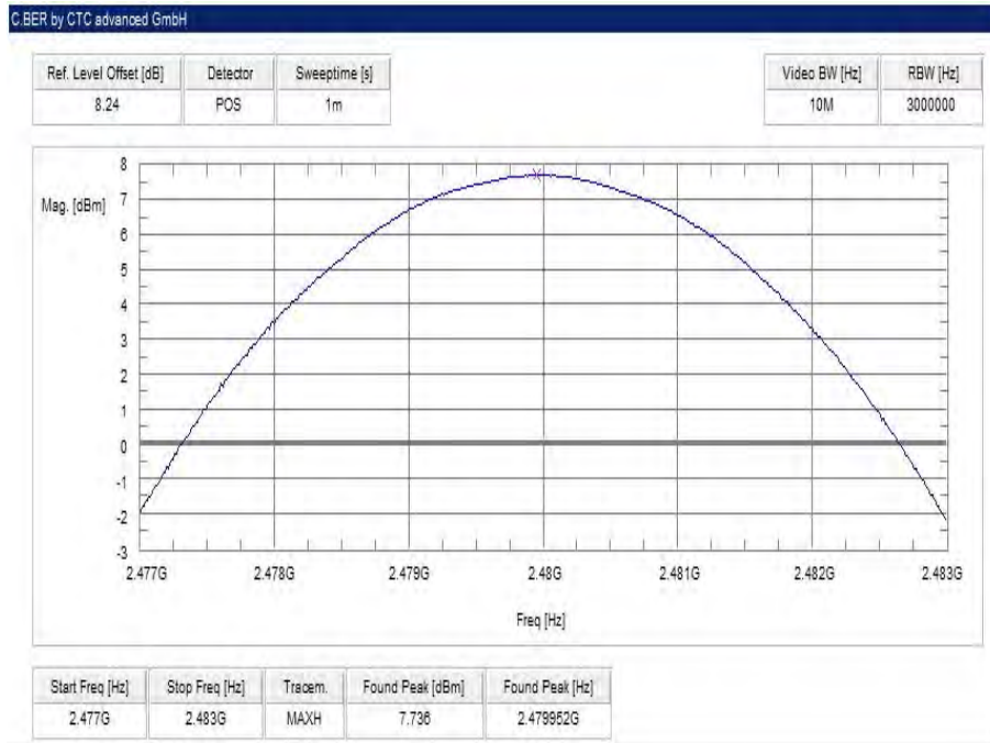
Plot 9: highest channel – 2480 MHz, 8 DPSK modulation
