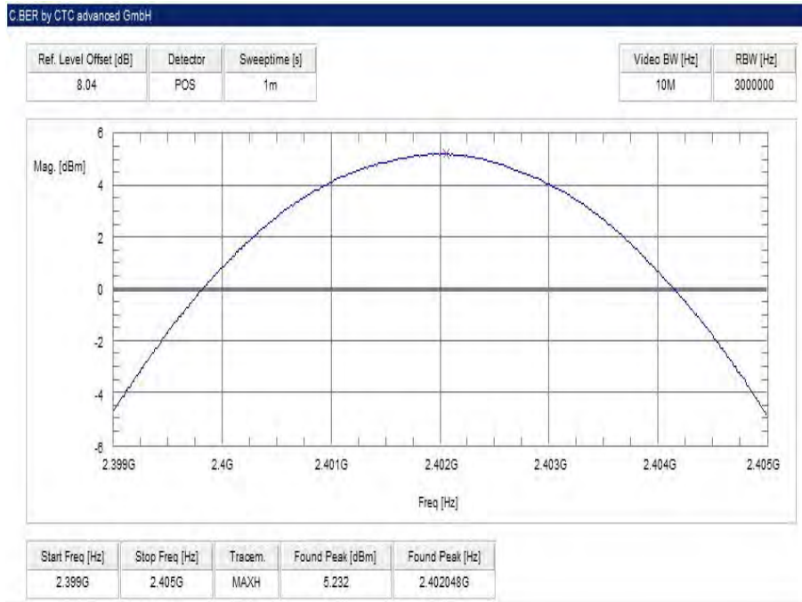
Plot 7: lowest channel – 2402 MHz, 8 DPSK modulation
