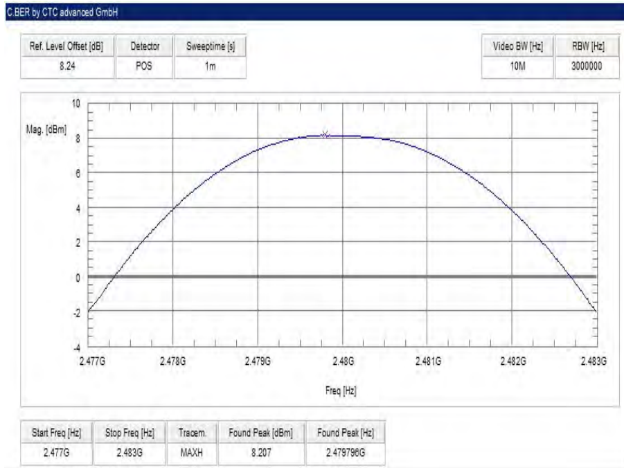
Plot 3: highest channel – 2480 MHz, GFSK modulation
