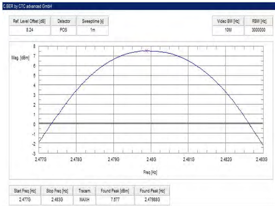
Plot 6: highest channel – 2480 MHz, Pi / DQPSK modulation
