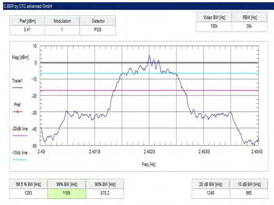
Plot 4: lowest channel – 2402 MHz, Pi / DQPSK modulation
