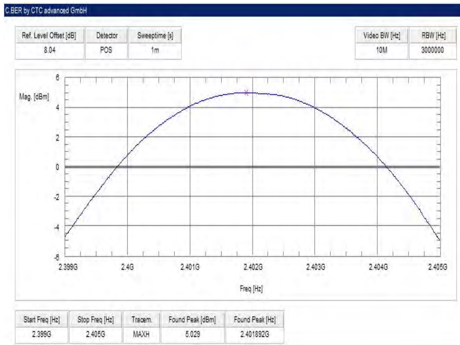
Plot 4: lowest channel – 2402 MHz, Pi / DQPSK modulation
