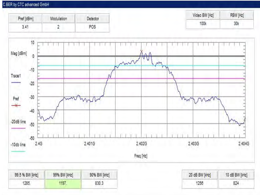
Plot 7: lowest channel – 2402 MHz, 8 DPSK modulation
