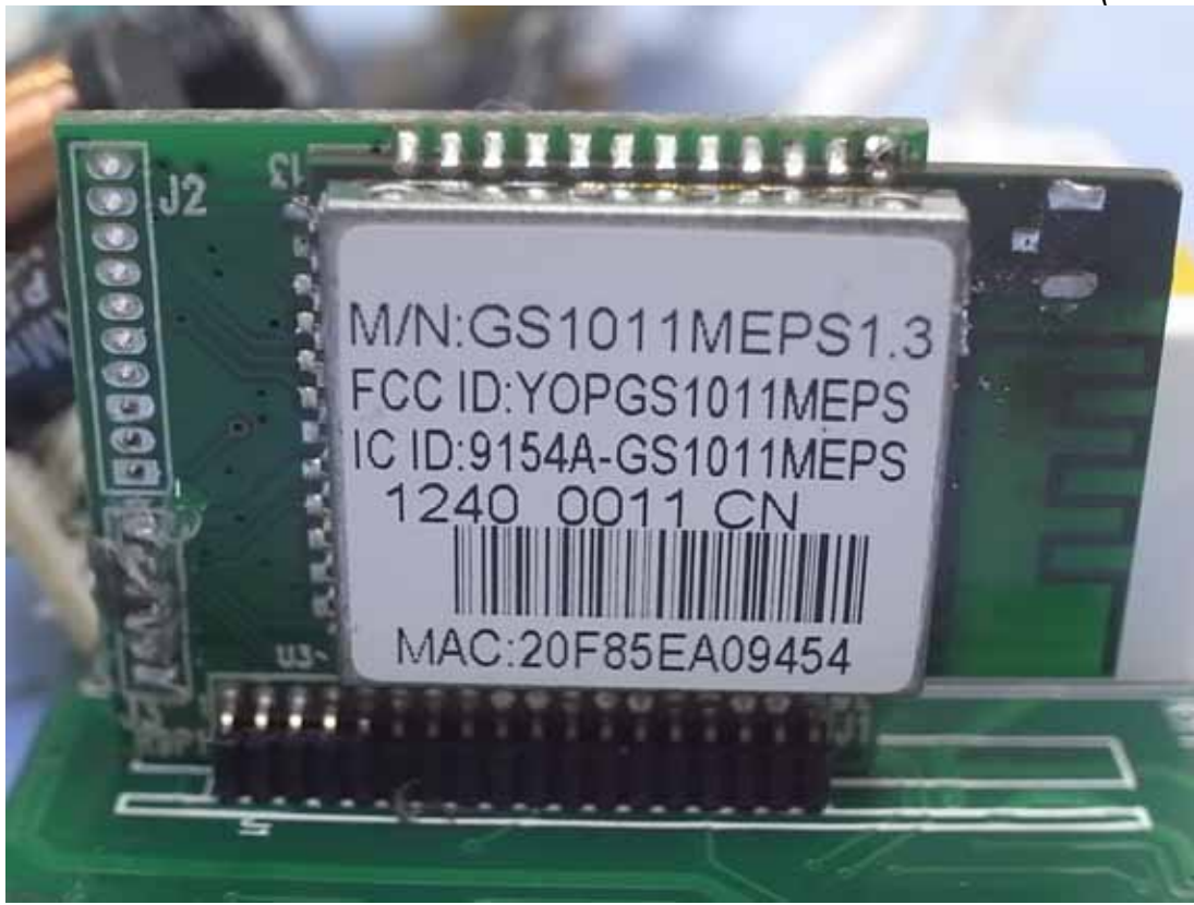
Photo 9 Internal View (Wi-Fi Module)
