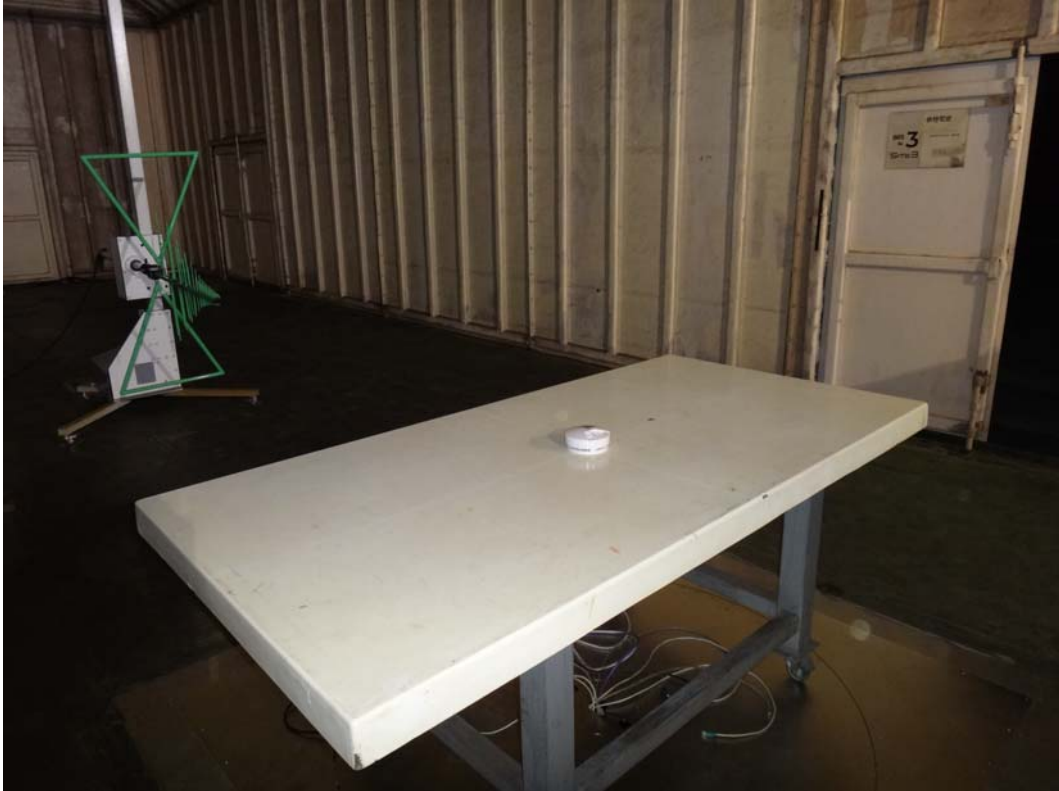
Front View of Radiated Test
