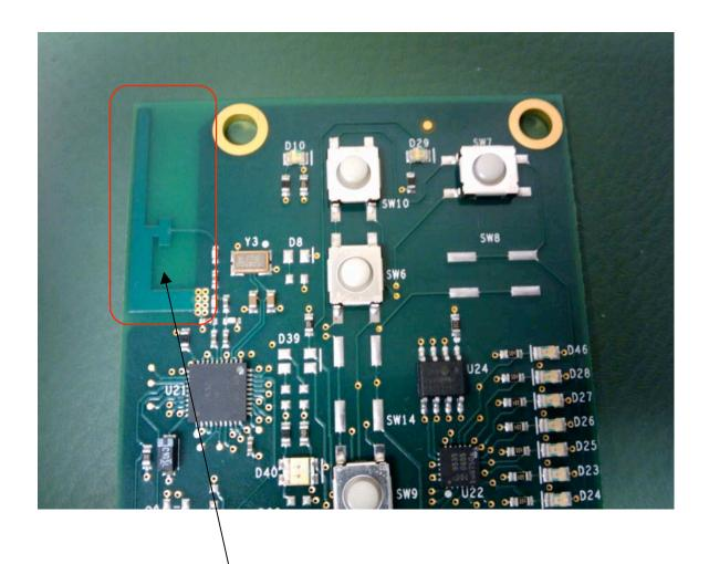
Location for mounting test antenna for EMI testing
