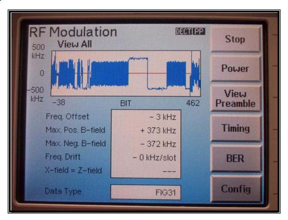
b) Carrier Frequency Stability over temperature
