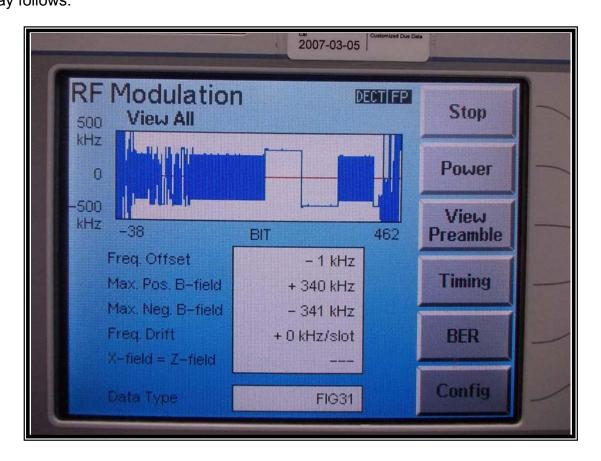
b) Carrier Frequency Stability over temperature
