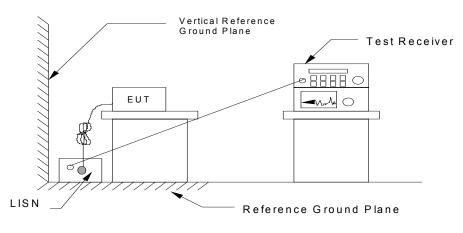
Test Set-Up 4
