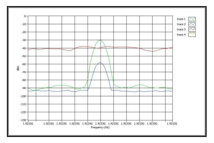
Comment1: Trace1 (green) is the interference on all 5 carriers. The level is Tu+UM+10dB. Comment2: Trace2 (blue) is interference on all 5 carriers. The level is TuR. Comment3: Trace3 (Red) is the EUT begins to transmit the beacon when interference level is TuR. Comment: 7.3.3b
