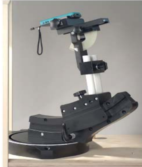
Fig. 9 Device holder supplied by SPEAG
