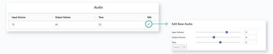
When using the PageFirst sensor, adjusting the sensitivity of the system can be done in the Base Details page. Click the edit icon to adjust the sensitivity level. Setting the sensitivity to 0 will disable this feature.
