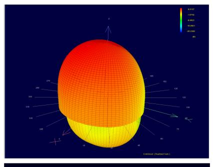
Bi-section 0.00° Amplitude Cut (Realized Gain)
