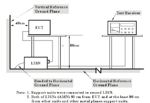
The setup of EUT is according with per ANSI C63.10-2013 measurement procedure. The specification used was with the FCC 15.315 and FCC 15.207 limits.
