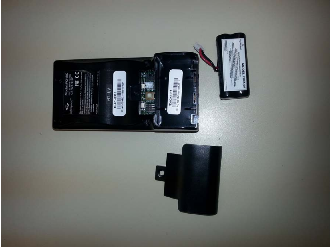
Battery Compartment of the FCHRC
