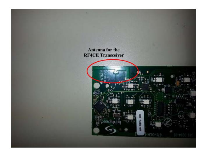
FRHRCB Antenna for the RF4CE Transceiver: Complies with FCC requirements per 15.203
