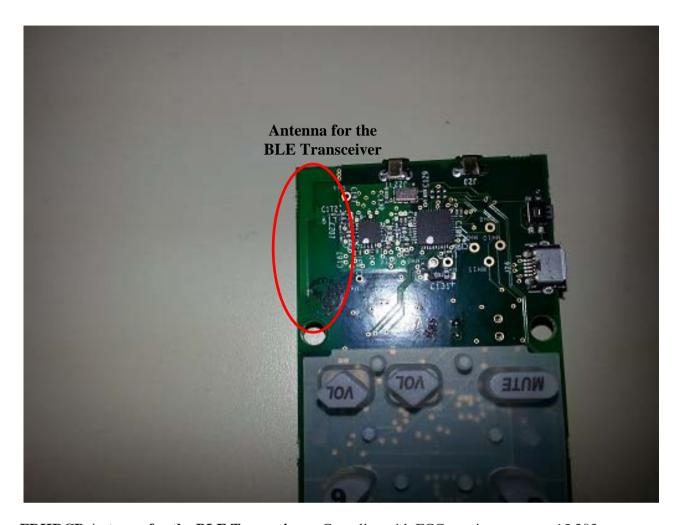
FRHRCB Antenna for the BLE Transceiver: Complies with FCC requirements per 15.203
