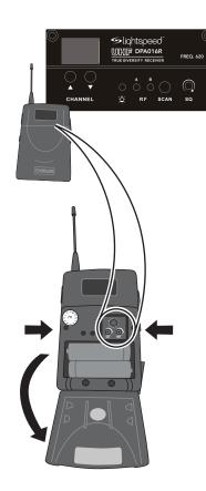
Transmitters and receivers are available in 3 different frequency groups (620, 645, 670 MHz). Verify that the frequency group of the receiver matches the letter code on the silver sticker in the battery compartment of the transmitter.
