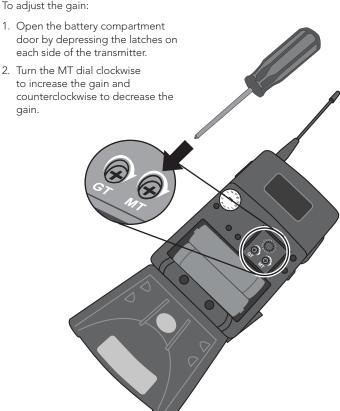
NOTE: If you are using a high impedance source, such as a guitar, it will be necessary to adjust the GT dial. Using a high impedance source requires a special cable. Contact Lightspeed Customer Service at 800-732-8999 for more information.
