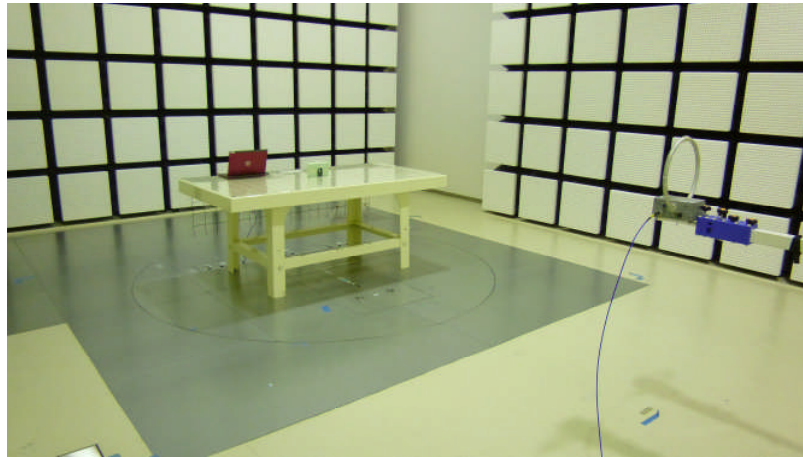
Photo1 Test setup for below 30 MHz ( Front )
