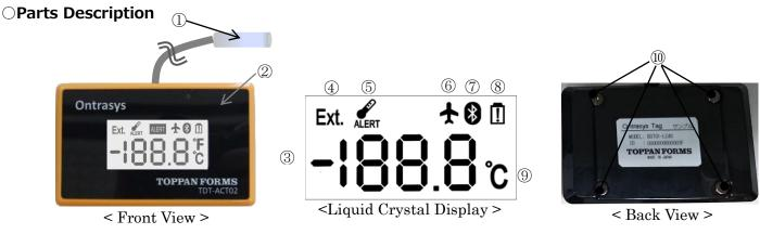
①External temperature sensor ②LED ③Temperature display ④External temperature ⑤Alert ⑥Airplane mode ⑦Usual mode ⑧Low battery alert ⑨℃ ⑩Mounting screws
