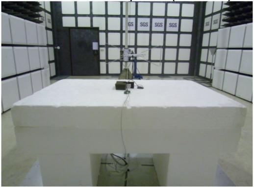
Radiated Emission Set up Photos (Above 1GHz)
