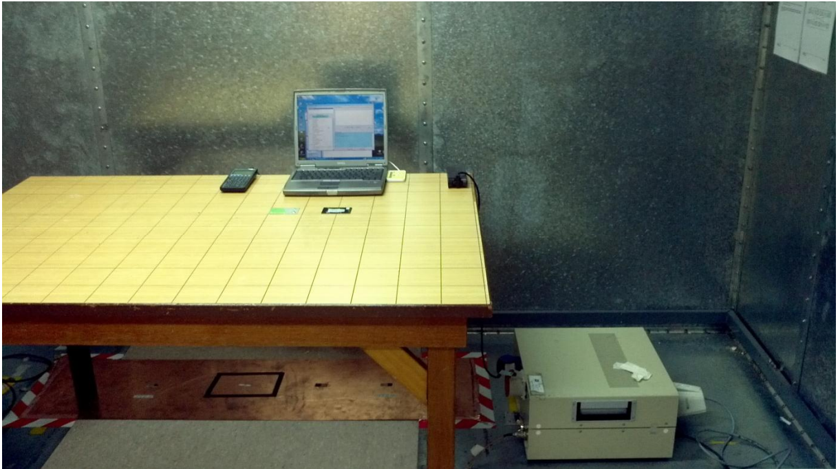
Conducted Emissions Test Setup (Front View)
