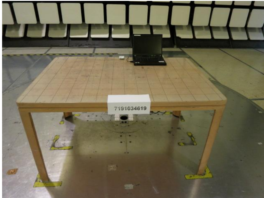
Radiated Emissions Test Setup (Front View)
