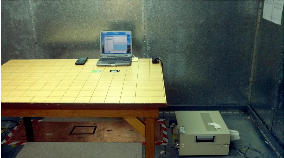
Conducted Emissions Test Setup (Front View)
