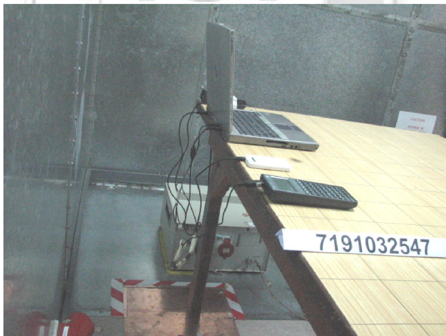
Conducted Emissions Test Setup (Rear View)
