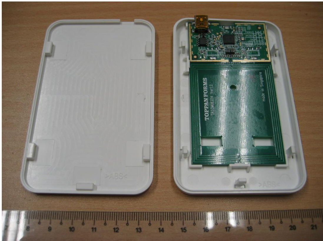
EUT Housing Internal View
