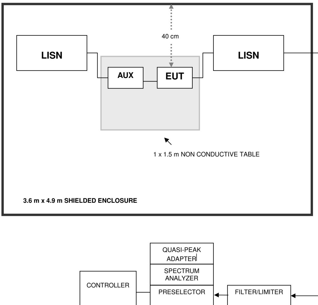
**FIGURE 2: Radiated Emissions Test Setup**
