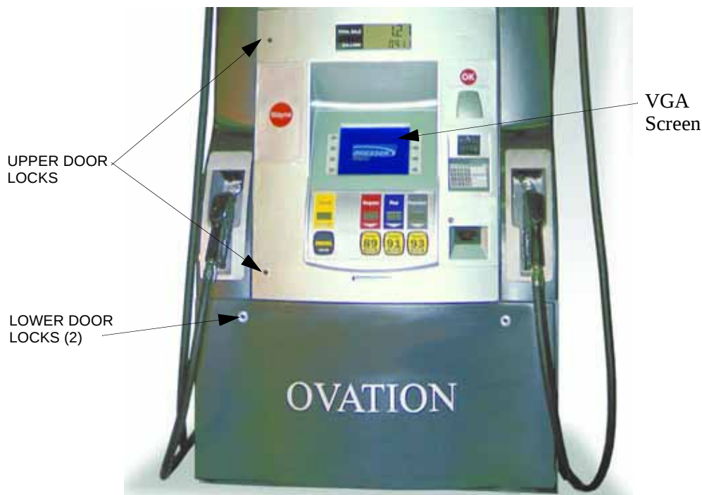
Figure 2-3 DOOR LOCK LOCATIONS. One door key fits upper and lower door locks. Optional VGA display screen shown.
