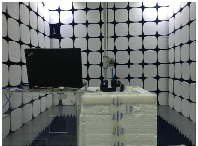
Radiated Spurious Emissions Test Setup Above
