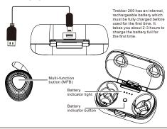
A. Put the headsets into the charging box and close the box to charge. During charging, the indicator shows a steady red. When the battery is fully charged, the red light will turn off.
