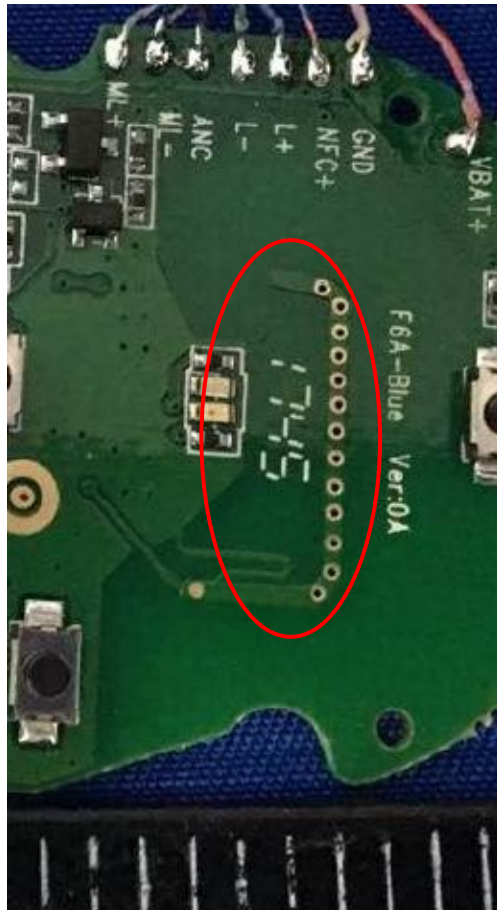
BT - Antenna View
