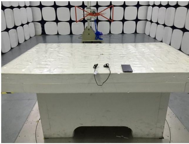
Radiated Spurious Emissions Test Setup Below 1GHz
