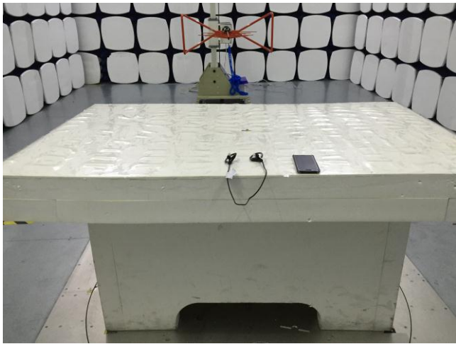
Radiated Spurious Emissions Test Setup Below 1GHz
