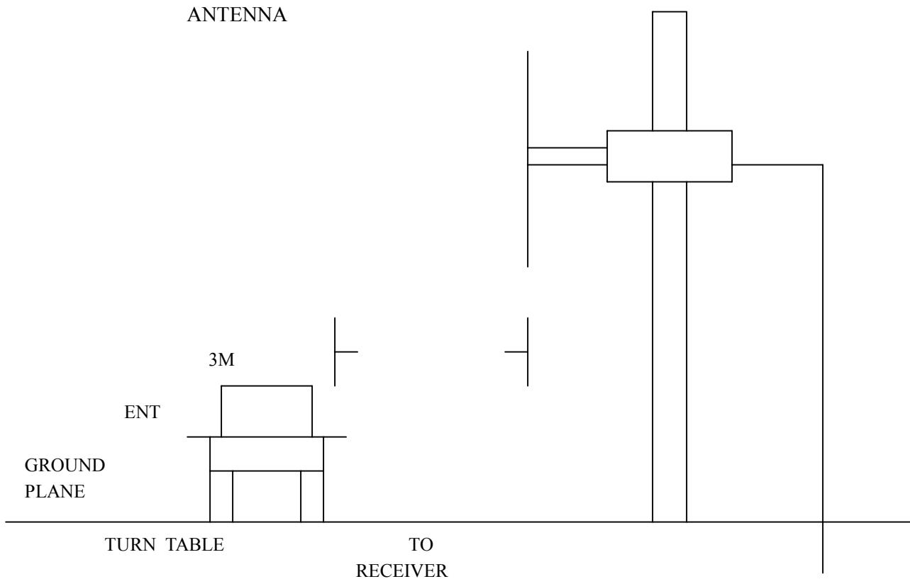
**4 . 3 RADIATED TEST SET-UP**
