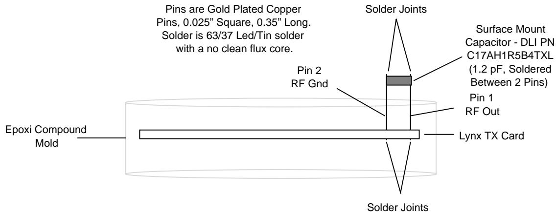
2. The design is limited to digital FSK modulation only. The 3<sup>rd</sup> paragraph is from standard Lynx documentation giving the capability of their device, however the analog FM capability is *not* supported in this application. As shown in the schematics of the TP-301 card, the data input into the Lynx TX is driven with a digital TTL interface, thus inhibiting the analog FM mode of operation. All test data and spectral provided were based on the digital FSK mode of operation.
