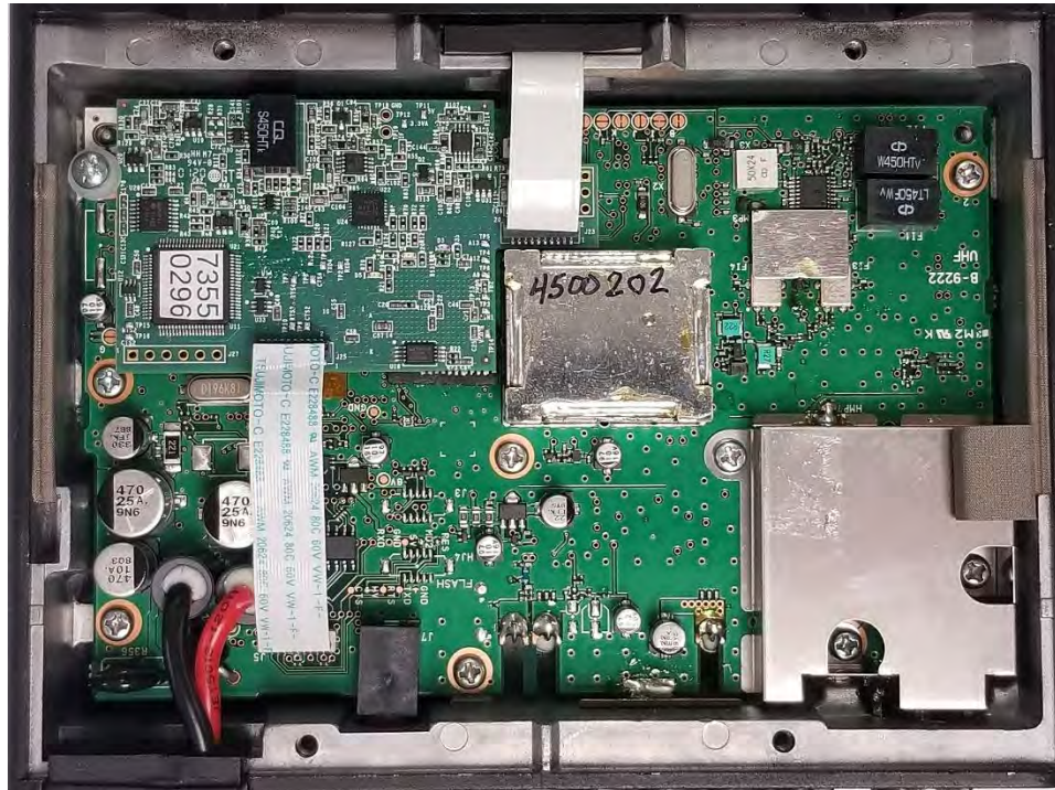
Main Board, Top, Shields Removed
