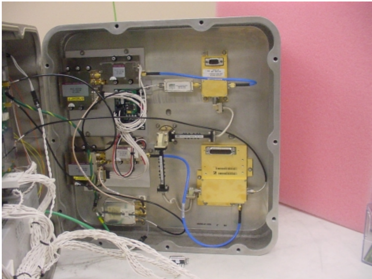
Internal photograph of transmitter, receiver, synthesizer, and filter/attenuator section
