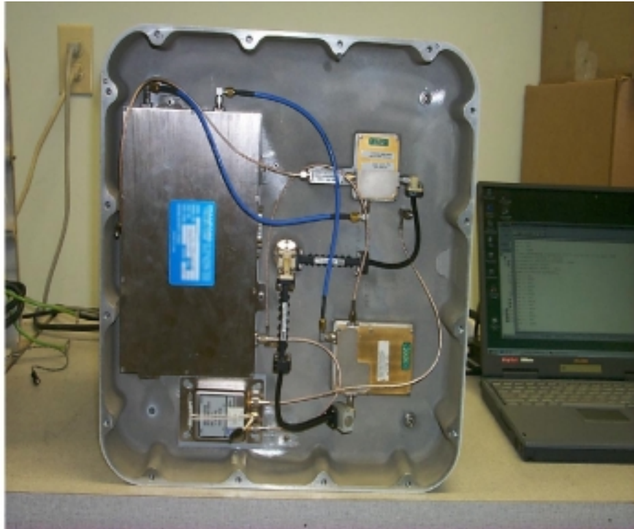
Internal photograph of transmitter, receiver, synthesizer, and filter/attenuator section
