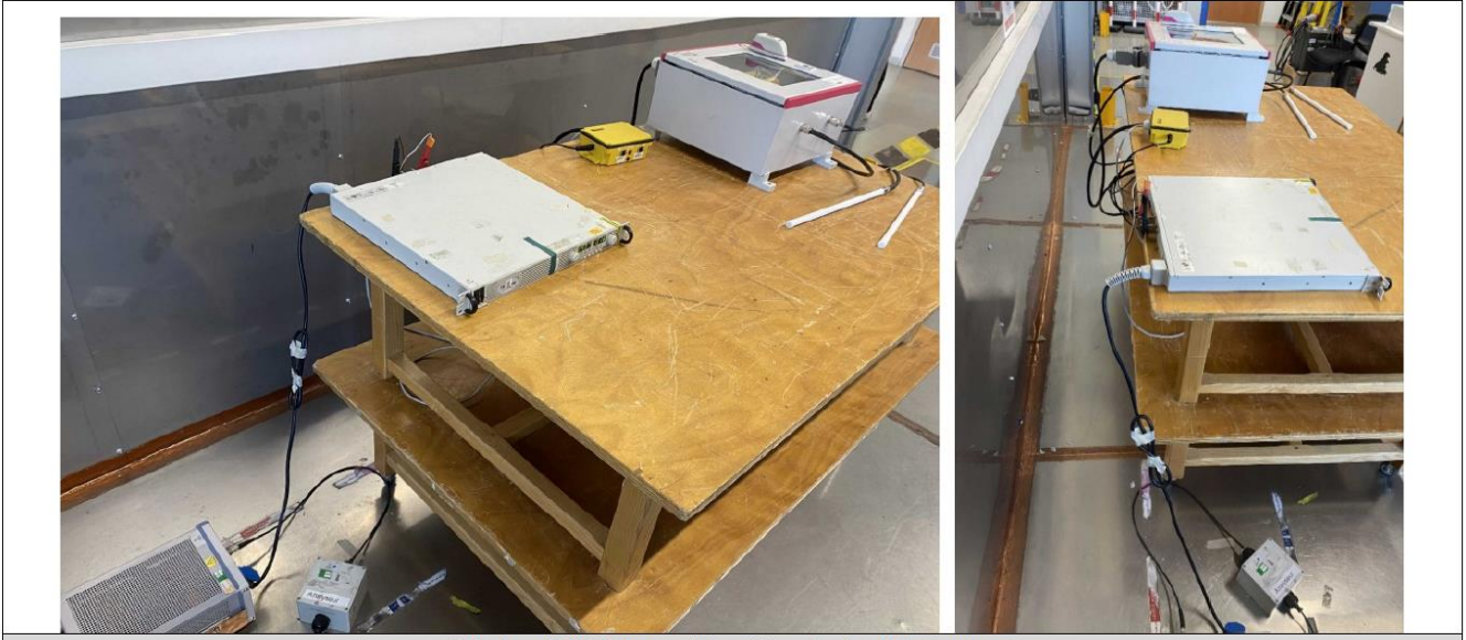
Photo of AC Power Line Conducted Emissions
