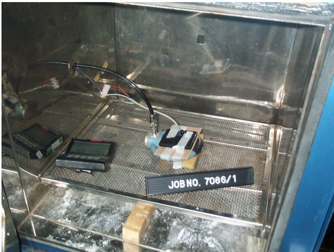
Fundamental supply voltage stability test.
