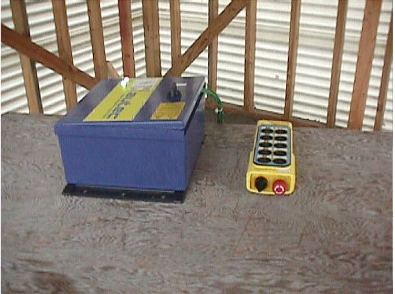
Photograph of Radiated Emissions Test Configuration
