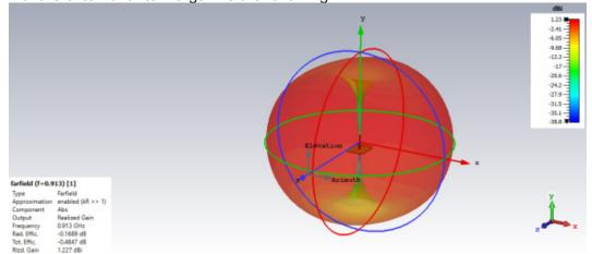
By simulation, as this diagram reports, the realized gain of the antenna is 1.227dBi and the System Total efficiency is -0.4847dB.
