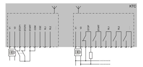
Example of wiring for command transmission working applications (machines which lift and transport material)
