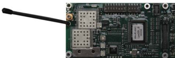
TOP VIEW OF TRANSMITTER BOARD CODE E16STXUS1
