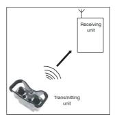
The MJ contains E16STXUS1. It is the radio transmitting module.
