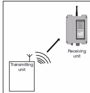
The receiving unit contains MRXUS06B. It is the radio receiving module.
