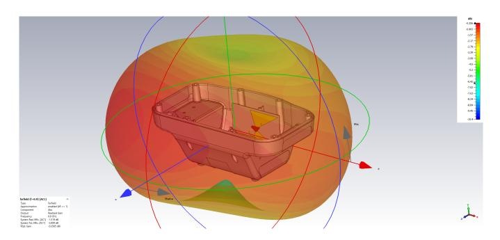
By simulation, as this diagram reports, the realized gain of the antenna is -0.3565dBi and the System Total efficiency is -2.009dB.
