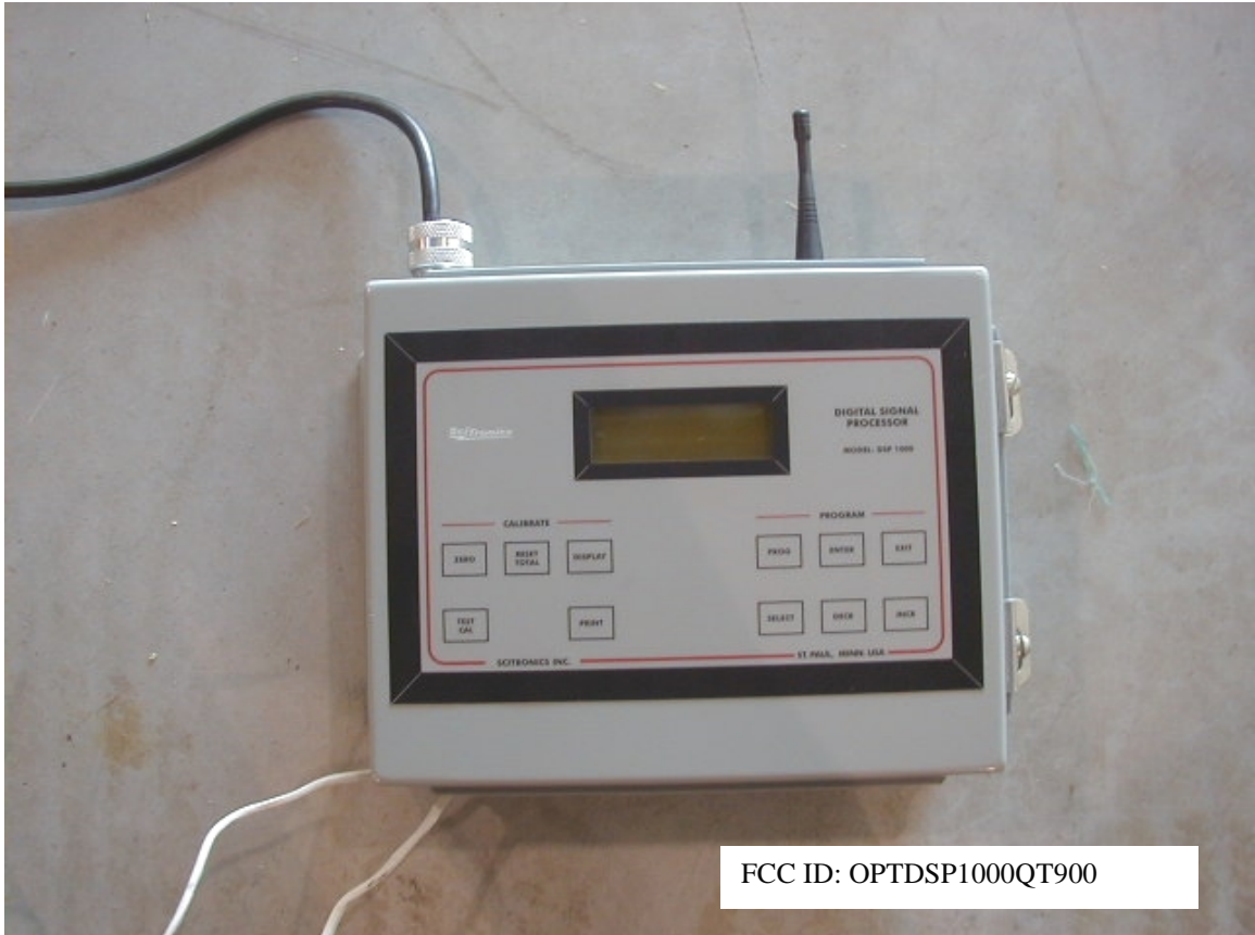
External Photo of Transmitter
