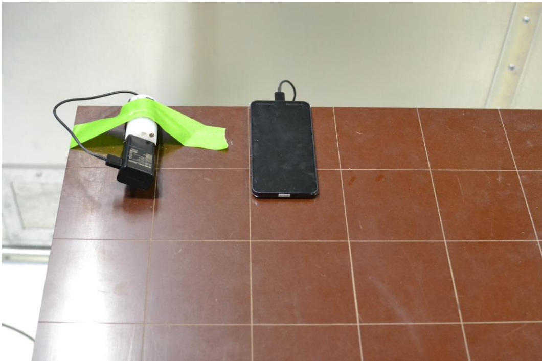
Figure 2. Test Setup – ACLC– <30MHz
