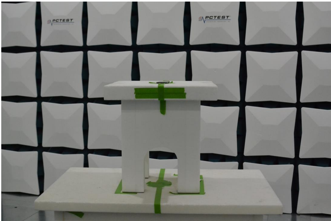
Figure 10. Test Setup – X Position – 1GHz-18GHz
