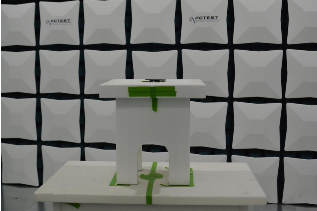
Figure 23. Test Setup – WPT Position – 1GHz-18GHz
