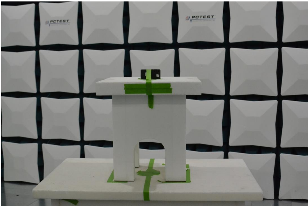
Figure 12. Test Setup – Y Position – 1GHz-18GHz
