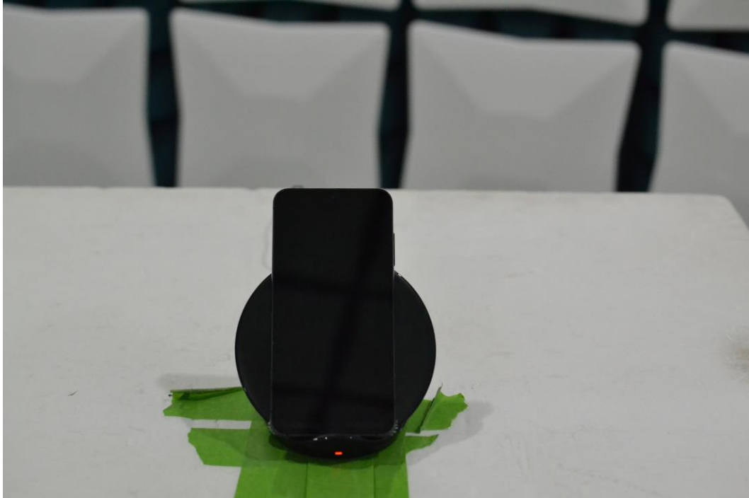
Figure 15. Test Setup – WCP Position – 1GHz-18GHz
