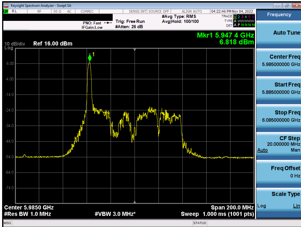
Plot 7-253. Power Spectral Density Plot MIMO ANT1 (80MHz BW 802.11ax (26 Tones) (UNII Band 5) – Ch. 7) – SP
