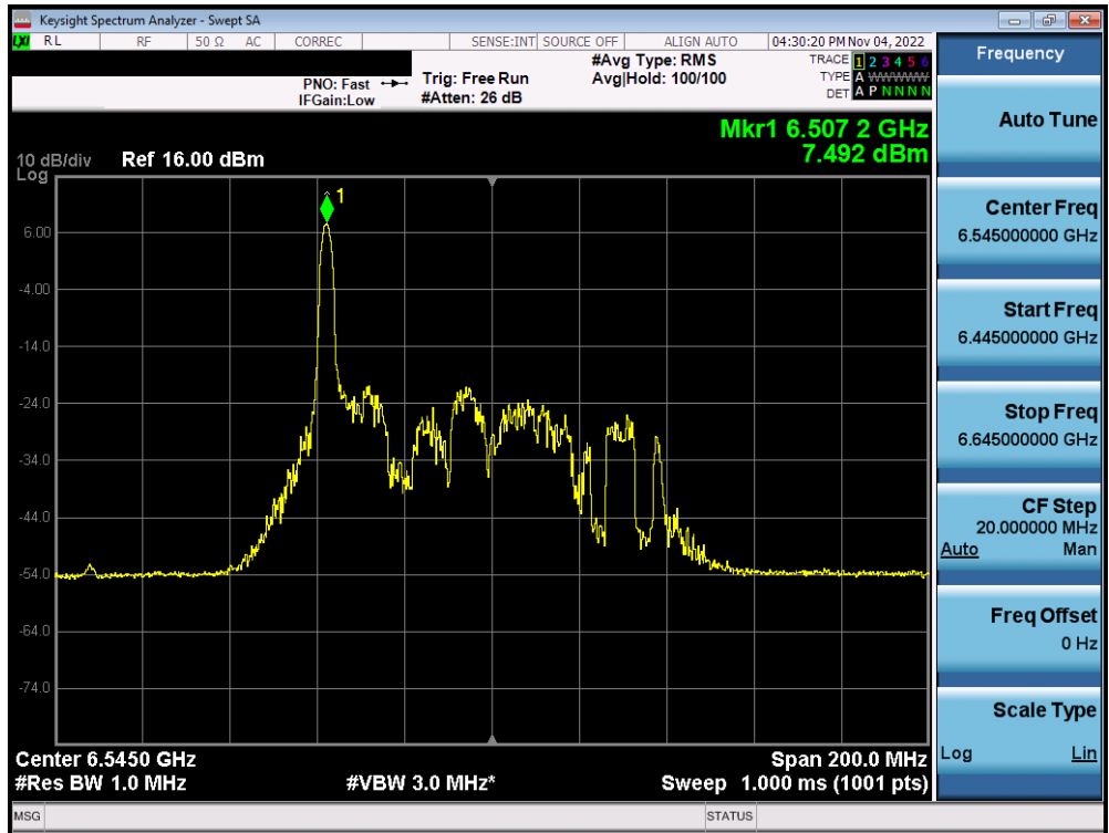
Plot 7-265. Power Spectral Density Plot MIMO ANT1 (80MHz BW 802.11ax (26 Tones) (UNII Band 7) – Ch. 119) – SP
