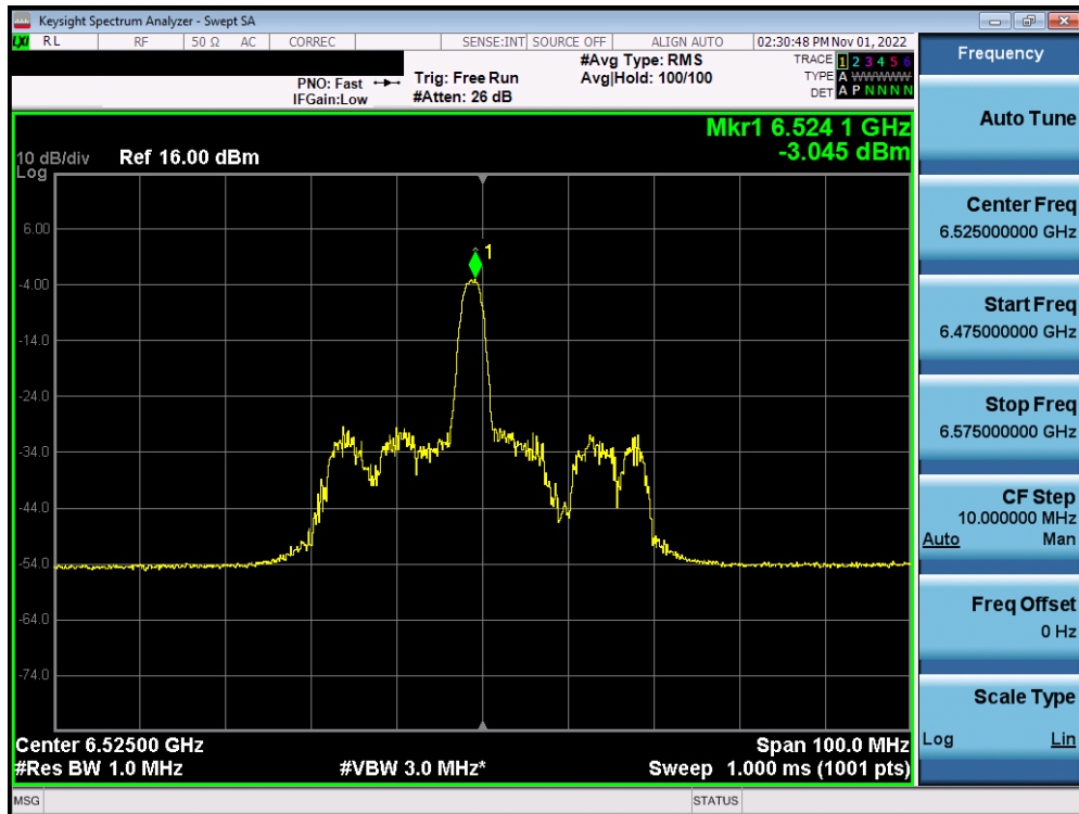
Plot 7-330. Power Spectral Density Plot MIMO ANT2 (40MHz BW 802.11ax (26 Tones) (UNII Band 6) – Ch. 115) – LPI
