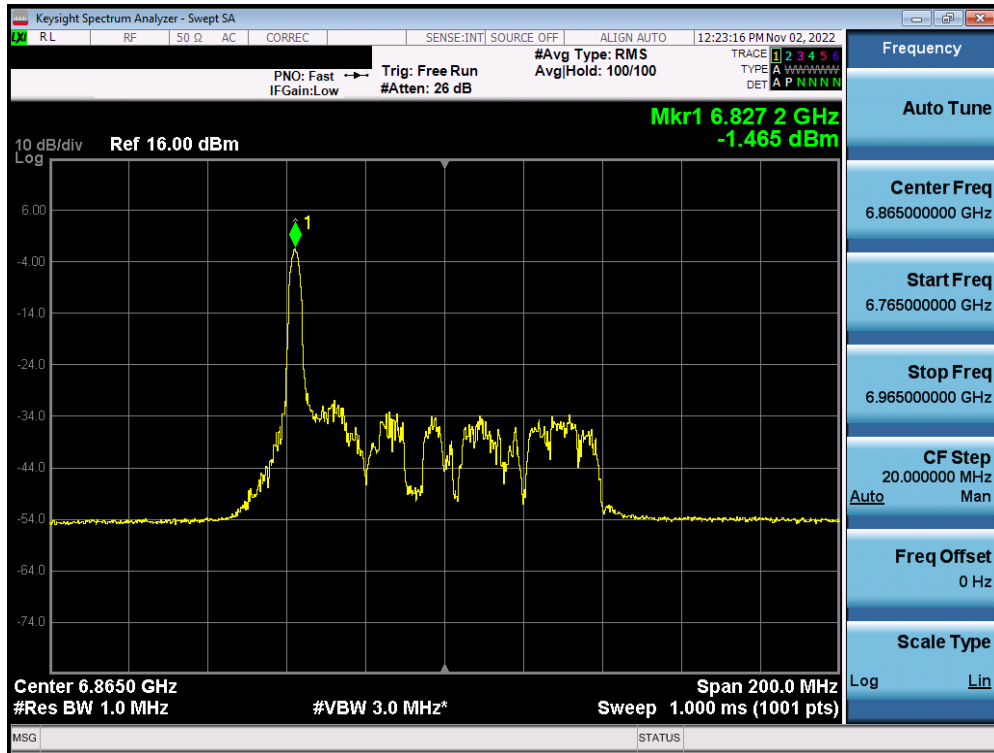
Plot 7-341. Power Spectral Density Plot MIMO ANT2 (80MHz BW 802.11ax (26 Tones) (UNII Band 7) – Ch. 183) – LPI
