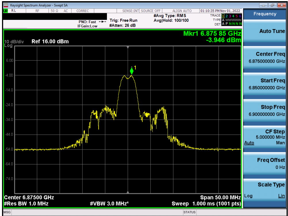
Plot 7-335. Power Spectral Density Plot MIMO ANT2 (20MHz BW 802.11ax (26 Tones) (UNII Band 7) – Ch. 185) – LPI
