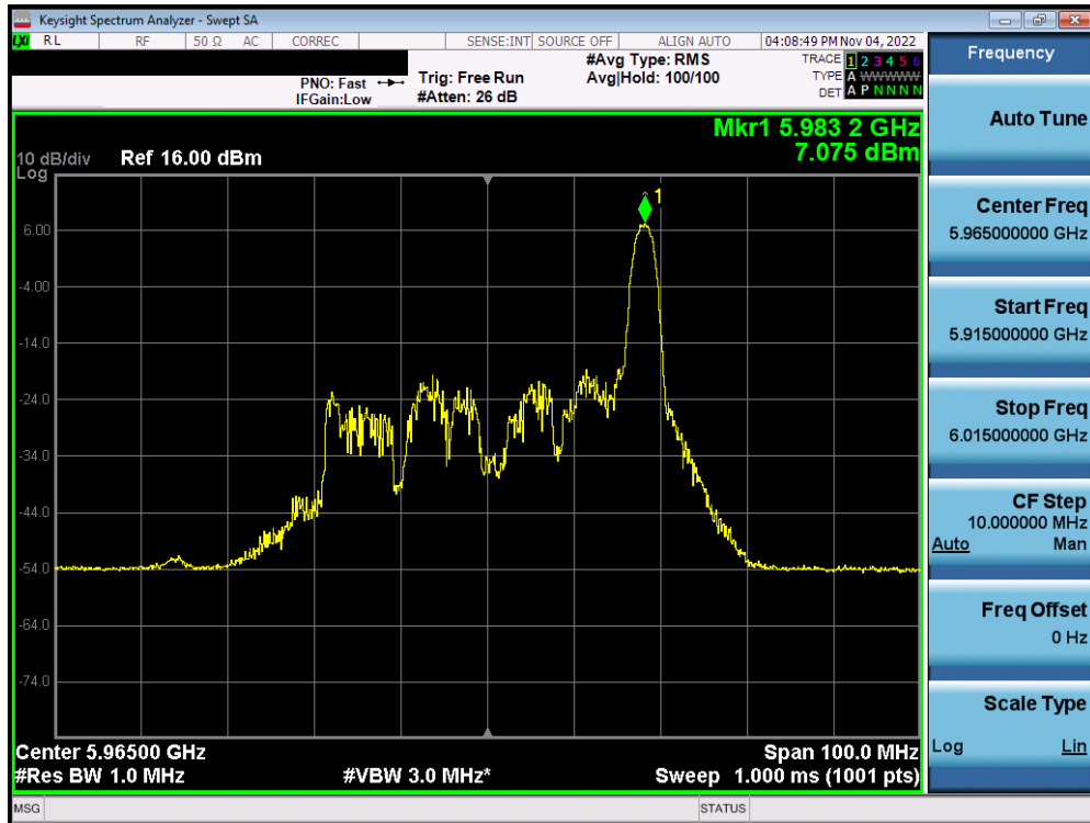
Plot 7-250. Power Spectral Density Plot MIMO ANT1 (40MHz BW 802.11ax (26 Tones) (UNII Band 5) – Ch. 3) – SP
