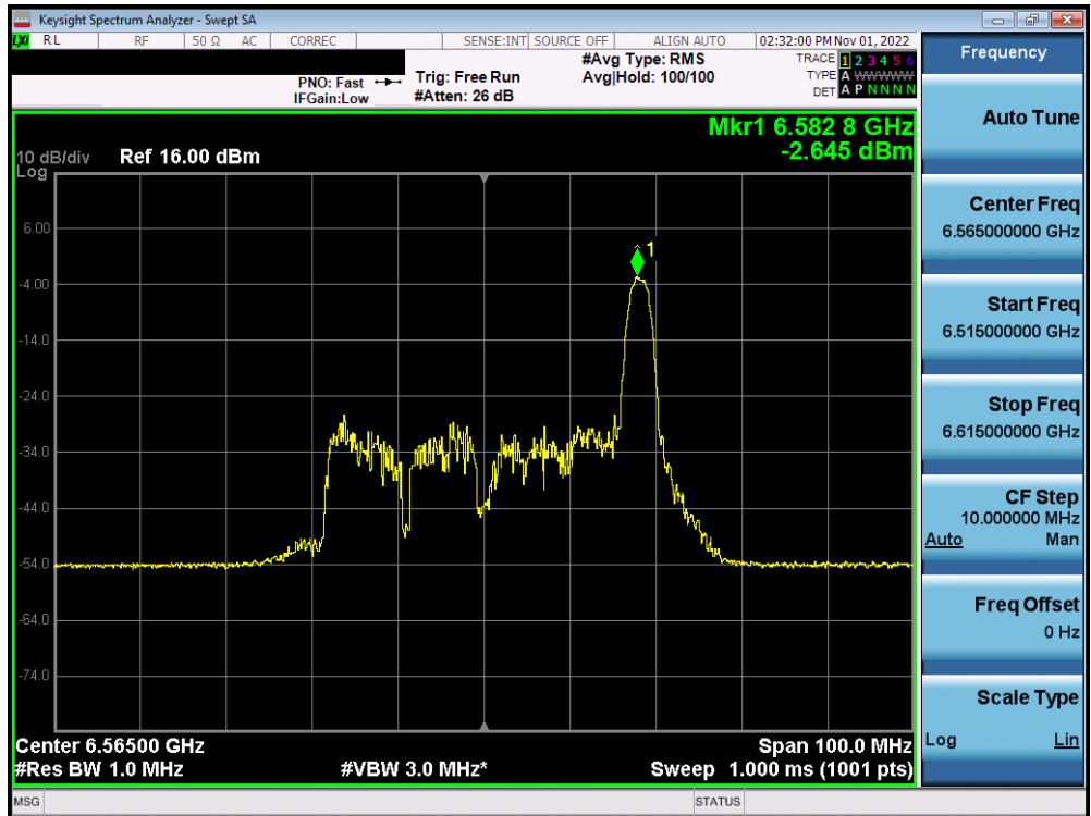
Plot 7-336. Power Spectral Density Plot MIMO ANT2 (40MHz BW 802.11ax (26 Tones) (UNII Band 7) – Ch. 123) – LPI
