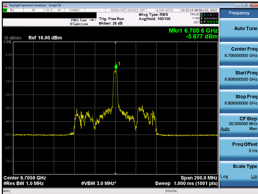
Plot 7-234. Power Spectral Density Plot MIMO ANT1 (80MHz BW 802.11ax (26 Tones) (UNII Band 7) – Ch. 151) – LPI
