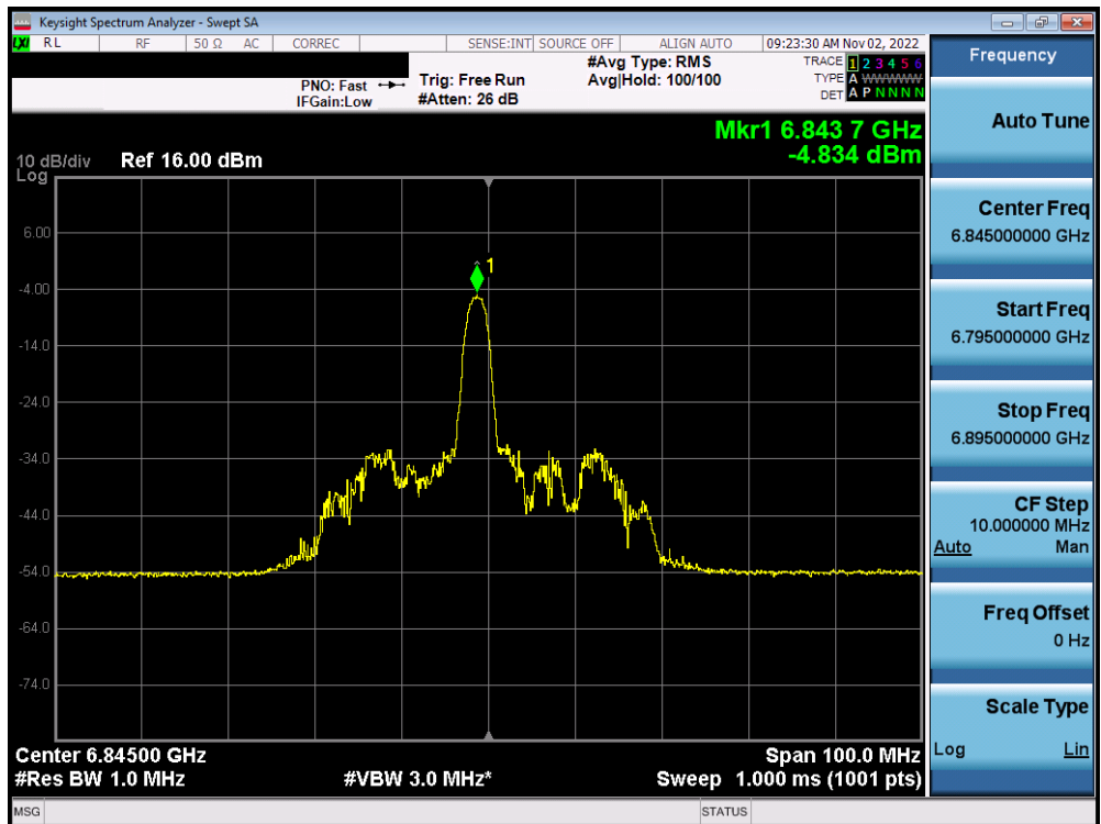
Plot 7-232. Power Spectral Density Plot MIMO ANT1 (40MHz BW 802.11ax (26 Tones) (UNII Band 7) – Ch. 179) – LPI
