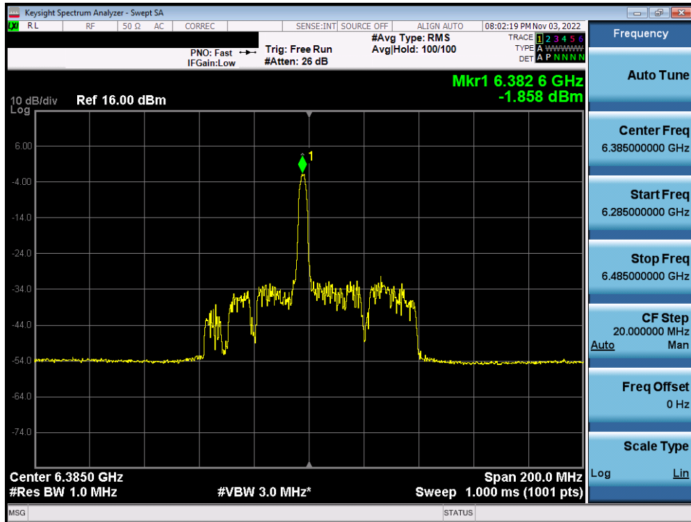
Plot 7-321. Power Spectral Density Plot MIMO ANT2 (80MHz BW 802.11ax (26 Tones) (UNII Band 5) – Ch. 87) – LPI
