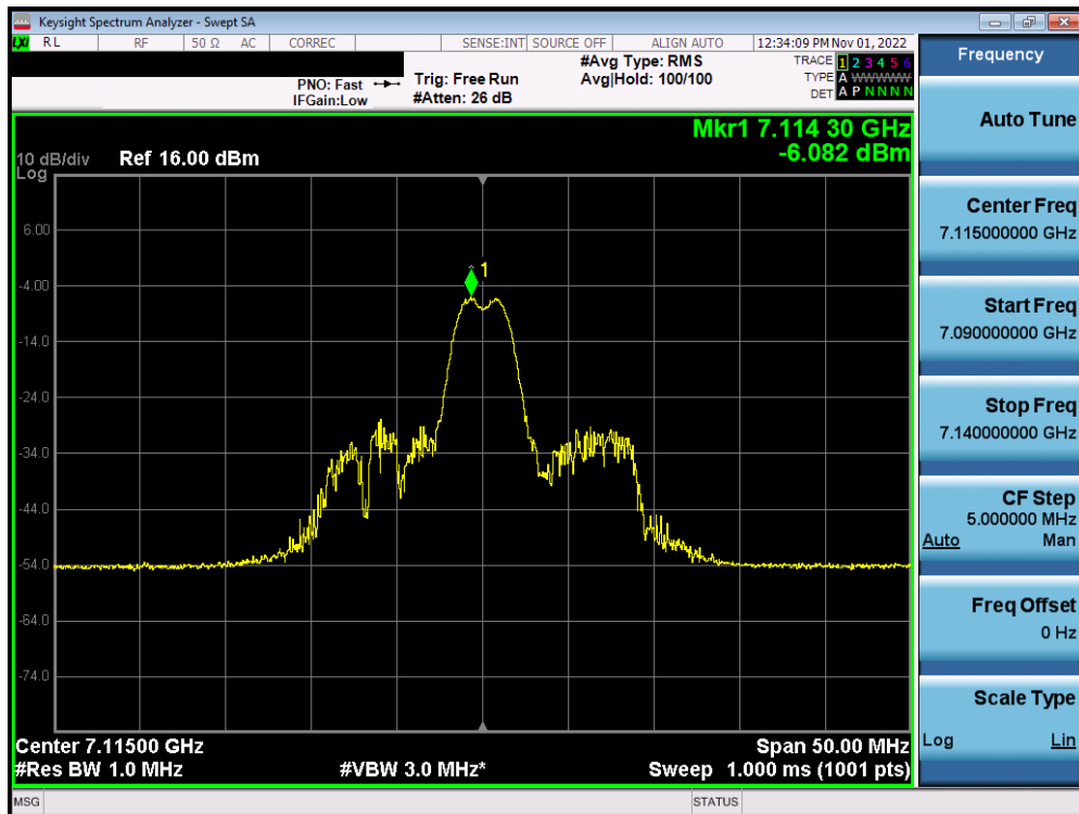
Plot 7-240. Power Spectral Density Plot MIMO ANT1 (20MHz BW 802.11ax (26 Tones) (UNII Band 8) – Ch. 233) – LPI
