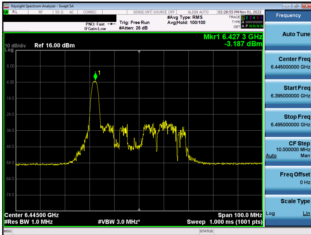
Plot 7-328. Power Spectral Density Plot MIMO ANT2 (40MHz BW 802.11ax (26 Tones) (UNII Band 6) – Ch. 99) – LPI
