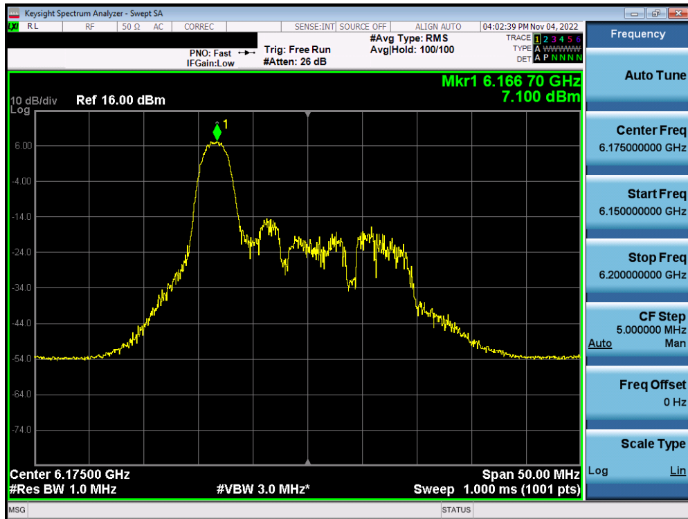
Plot 7-248. Power Spectral Density Plot MIMO ANT1 (20MHz BW 802.11ax (26 Tones) (UNII Band 5) – Ch. 45) – SP
