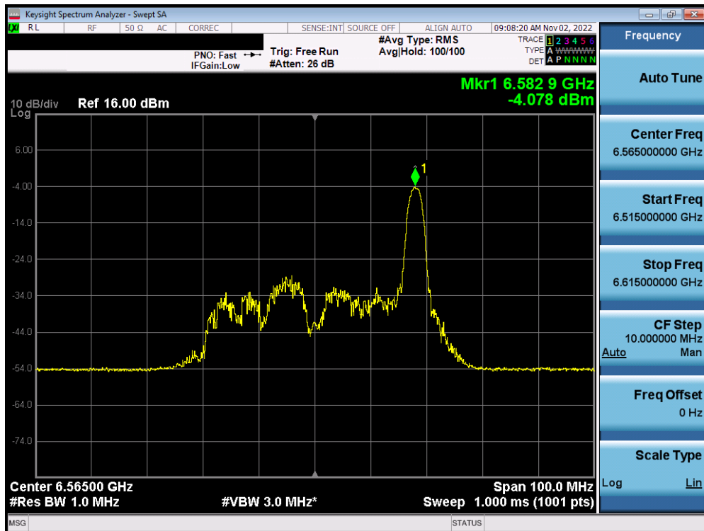
Plot 7-230. Power Spectral Density Plot MIMO ANT1 (40MHz BW 802.11ax (26 Tones) (UNII Band 7) – Ch. 123) – LPI
