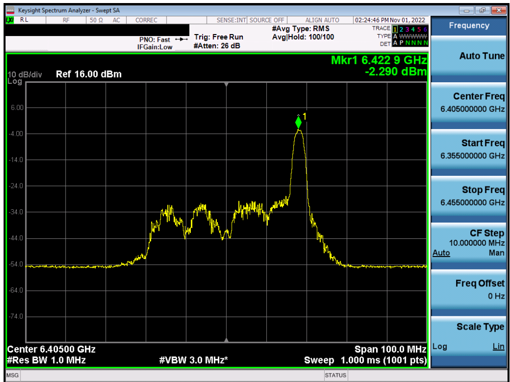
Plot 7-318. Power Spectral Density Plot MIMO ANT2 (40MHz BW 802.11ax (26 Tones) (UNII Band 5) – Ch. 91) – LPI
