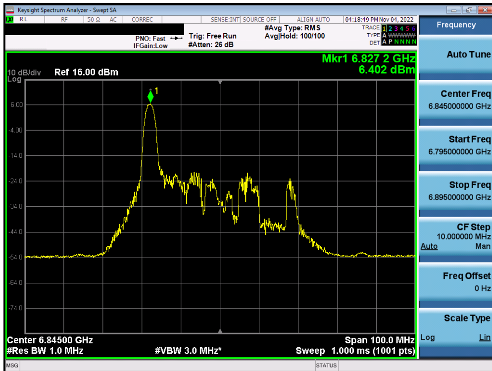
Plot 7-264. Power Spectral Density Plot MIMO ANT1 (40MHz BW 802.11ax (26 Tones) (UNII Band 7) – Ch. 179) – SP
