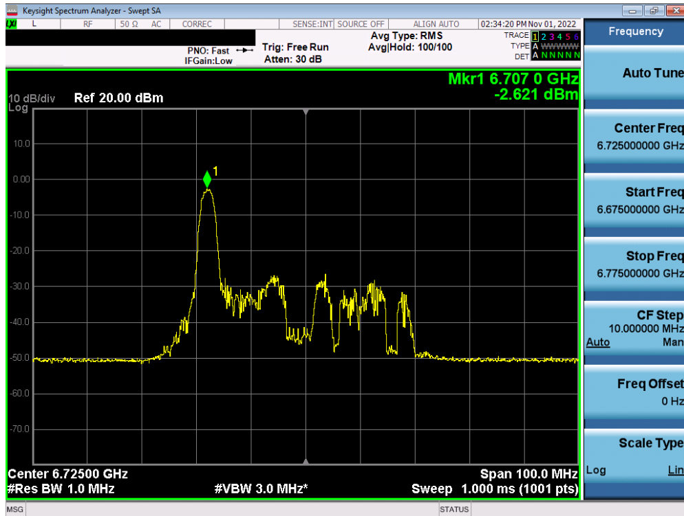
Plot 7-337. Power Spectral Density Plot MIMO ANT2 (40MHz BW 802.11ax (26 Tones) (UNII Band 7) – Ch. 155) – LPI
