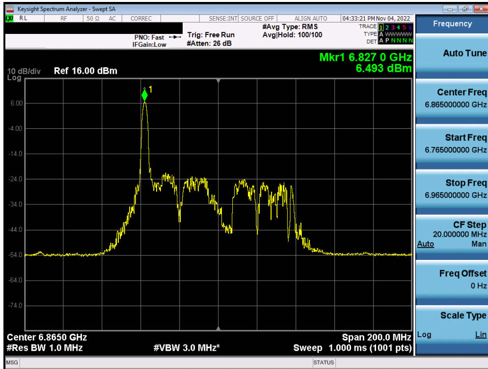
Plot 7-267. Power Spectral Density Plot MIMO ANT1 (80MHz BW 802.11ax (26 Tones) (UNII Band 7) – Ch. 183) – SP
