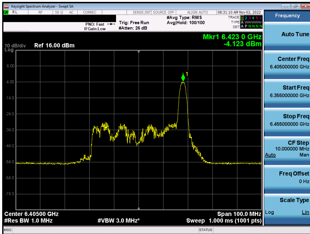
Plot 7-212. Power Spectral Density Plot MIMO ANT1 (40MHz BW 802.11ax (26 Tones) (UNII Band 5) – Ch. 91) – LPI
