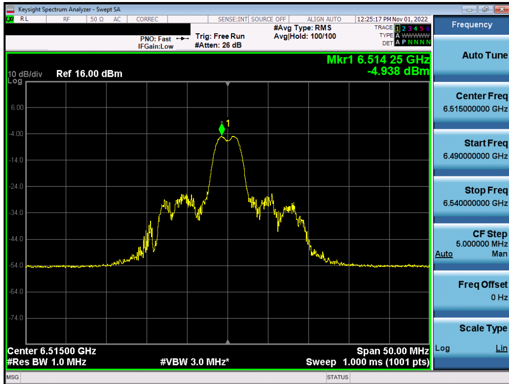
Plot 7-221. Power Spectral Density Plot MIMO ANT1 (20MHz BW 802.11ax (26 Tones) (UNII Band 6) – Ch. 113) – LPI
