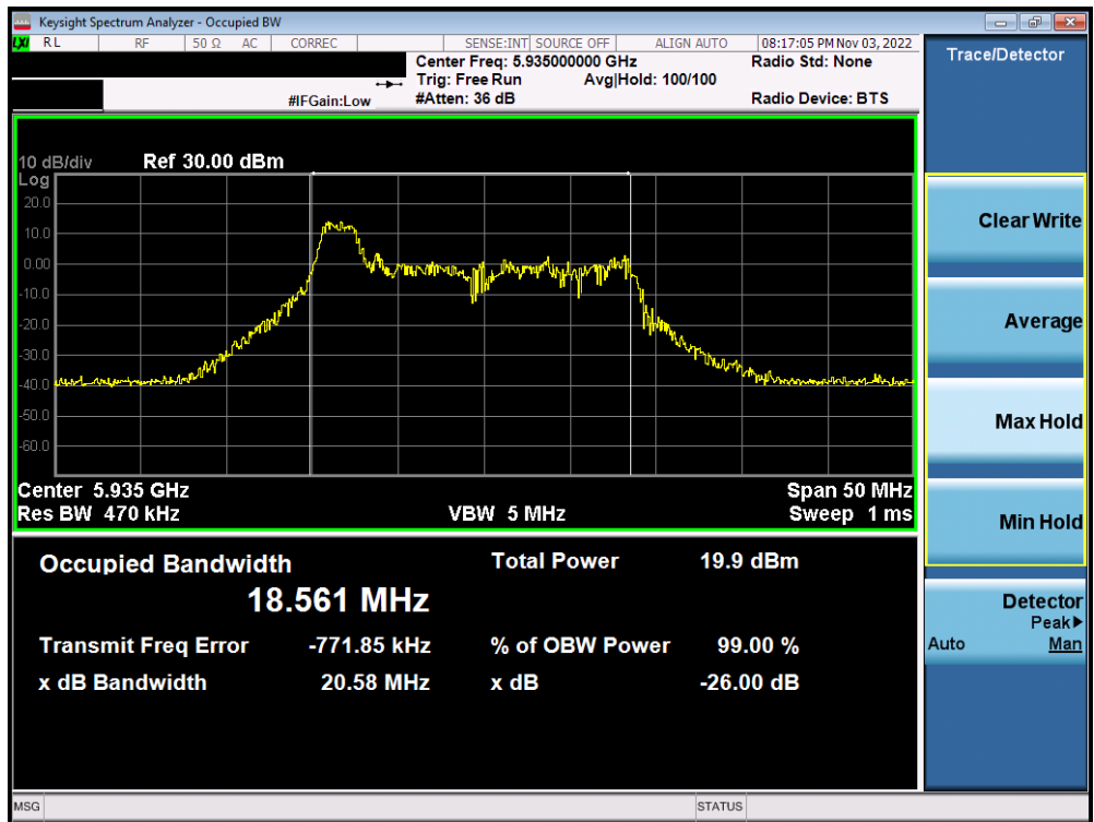
Plot 7-144. Occupied Bandwidth Plot MIMO ANT2 (20MHz BW 802.11ax (26 Tones) UNII Band 5) – Ch. 2 – SP
