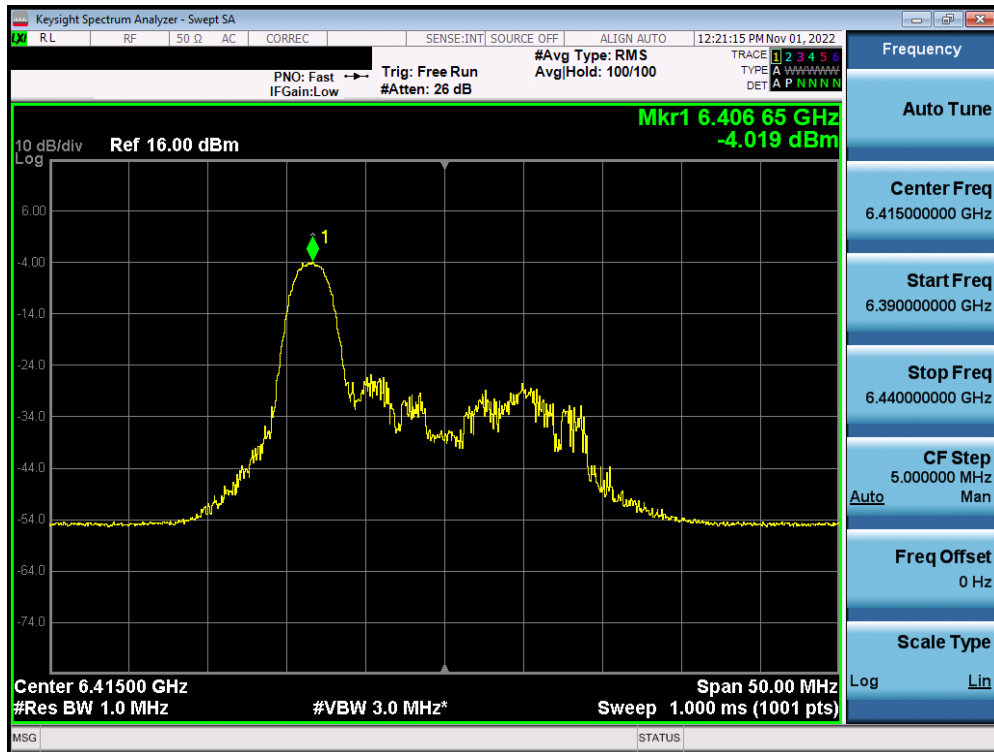
Plot 7-209. Power Spectral Density Plot MIMO ANT1 (20MHz BW 802.11ax (26 Tones) UNII Band 5) – Ch. 93) – LPI
