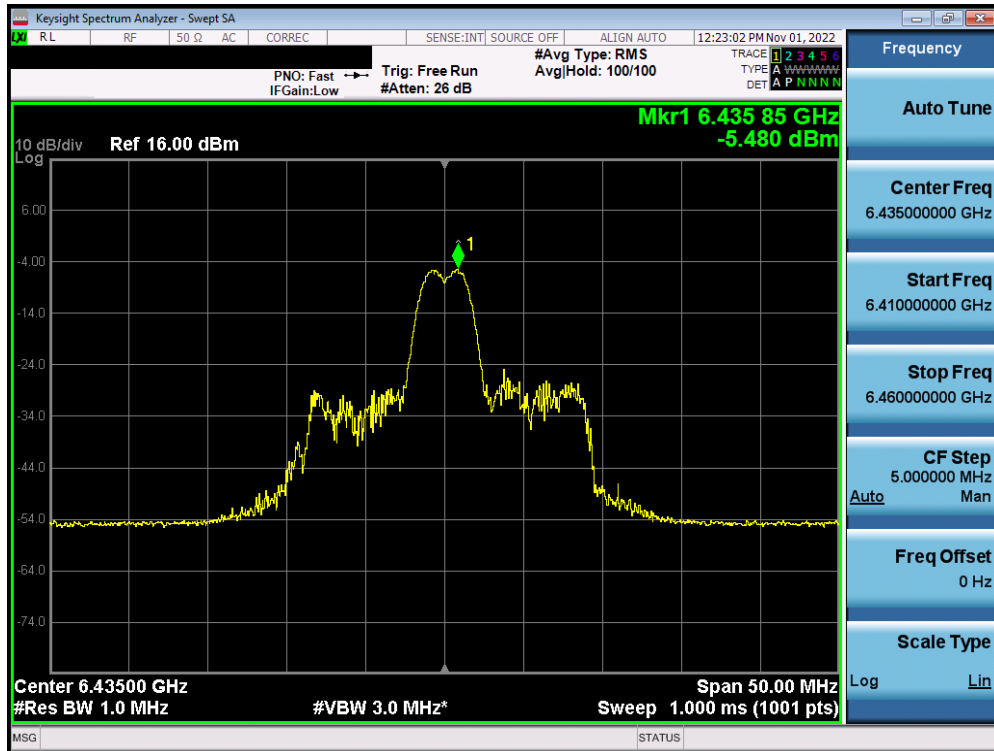
Plot 7-219. Power Spectral Density Plot MIMO ANT1 (20MHz BW 802.11ax (26 Tones) (UNII Band 6) – Ch. 97) – LPI
