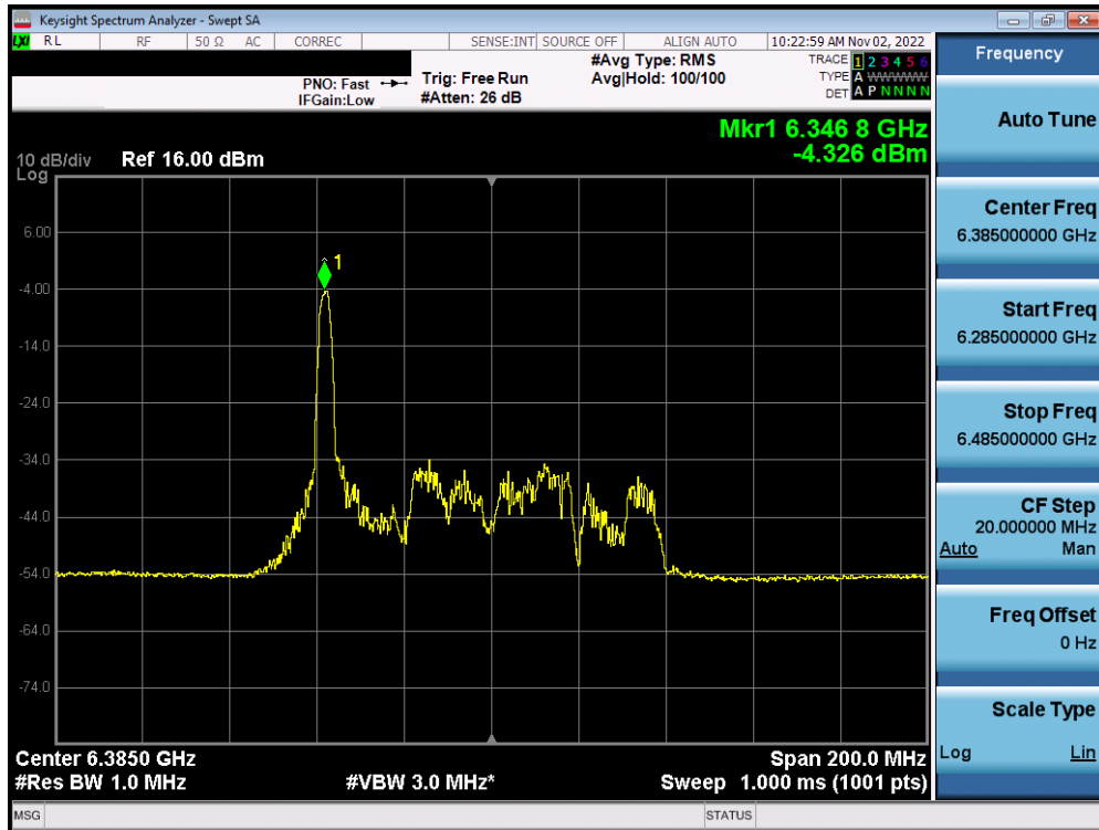
Plot 7-215. Power Spectral Density Plot MIMO ANT1 (80MHz BW 802.11ax (26 Tones) (UNII Band 5) – Ch. 87) – LPI
