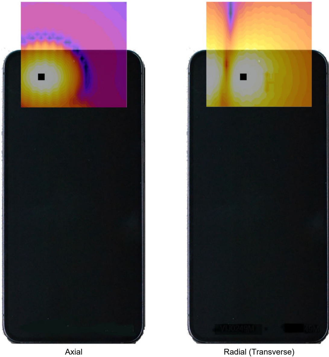
Figure 17-3 T-Coil Scan Overlay Magnetic Field Distributions
